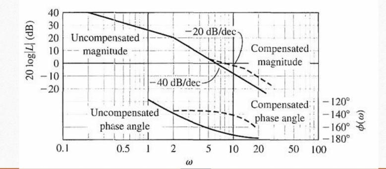
• The transfer function of the **phase-lag** network is *RC* **network** suitable for compensating a feedback control
