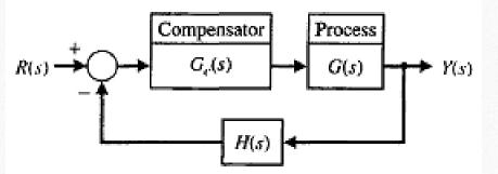
lead compensator for a system
