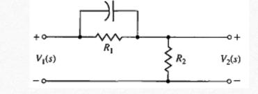
we obtain the **phase-lead compensation** transfer function  $G_{d}$ The maximum value of the phase lead occurs at a frequency  $\omega_m$ , The maximum phase lead occurs halfway between the pole and zero frequencies
